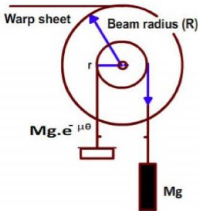
Figure 4.18: Warp tension control by dead weight system
