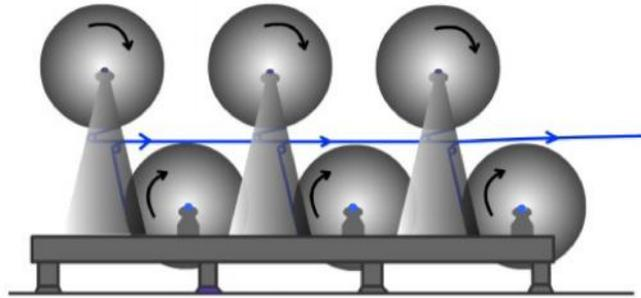
Figure 4.16: Equi-tension creel
