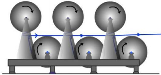
Figure 4.16: Equi-tension creel
