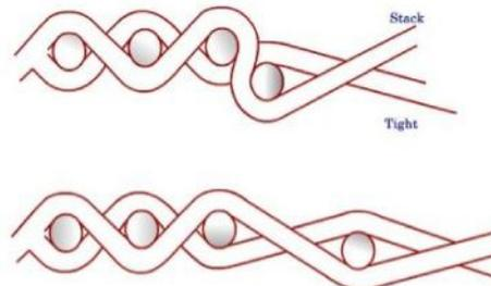
Figure 6.13. (a) Vertical displacement of newly inserted weft (b) Beat up at crossed shed
