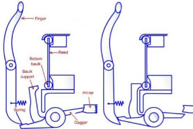
Figure 9.11: Loose-reed warp protector motion
