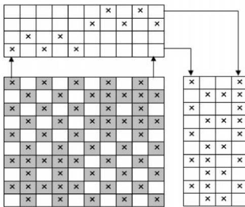
Figure 5.27: Design, drafting and lifting plan of Huck-a-back weave
