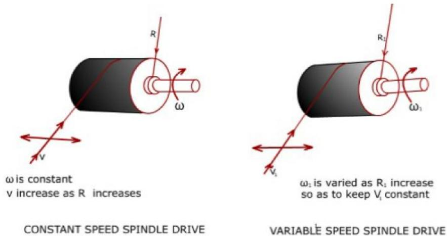
Figure 2.7: Spindle-driven winders
