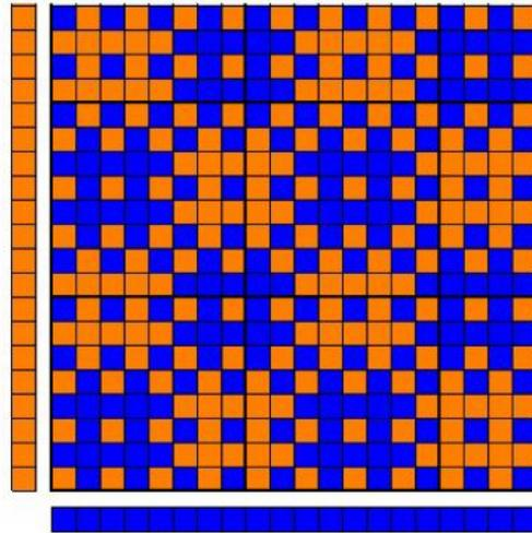
Figure 5.26: Extended view of the Mock leno weave
