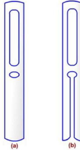
Figure 9.12: Drop wires
