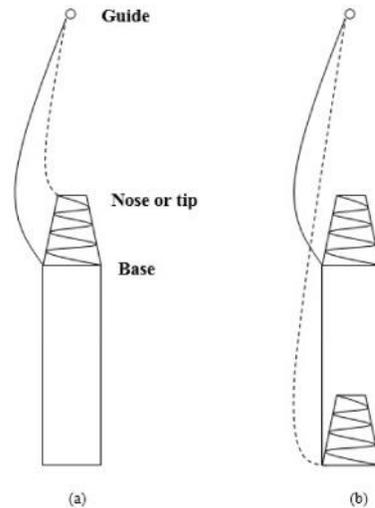
Figure 2.34: Short term and long term tension variation during unwinding
