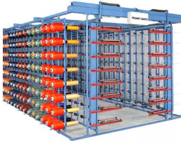
*Figure 3.2: A simple creel of warping machine*
