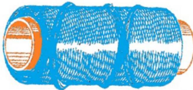
*Figure 2.49: Package with ribbon or pattern defect*
