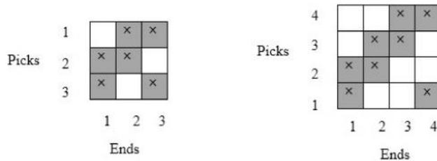
Figure 5.12: Warp faced (2/1) twill and balanced (2/2) twill
