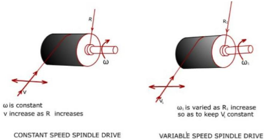
Figure 2.7: Spindle-driven winders
