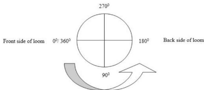
Figure 6.9: Different angular positions of crank shaft
