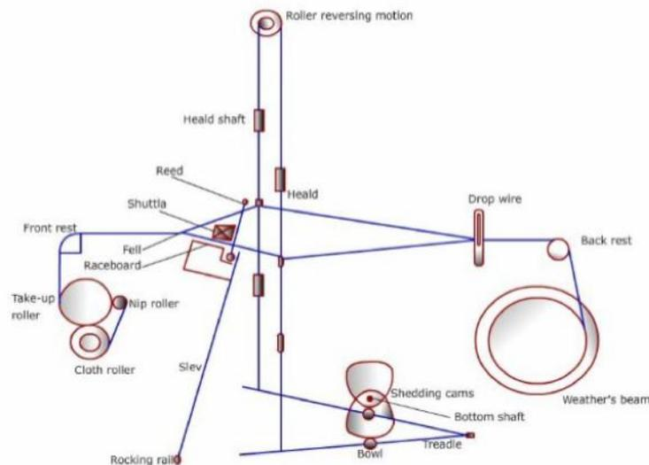
*Figure 6.2: Cross-sectional view of loom*
