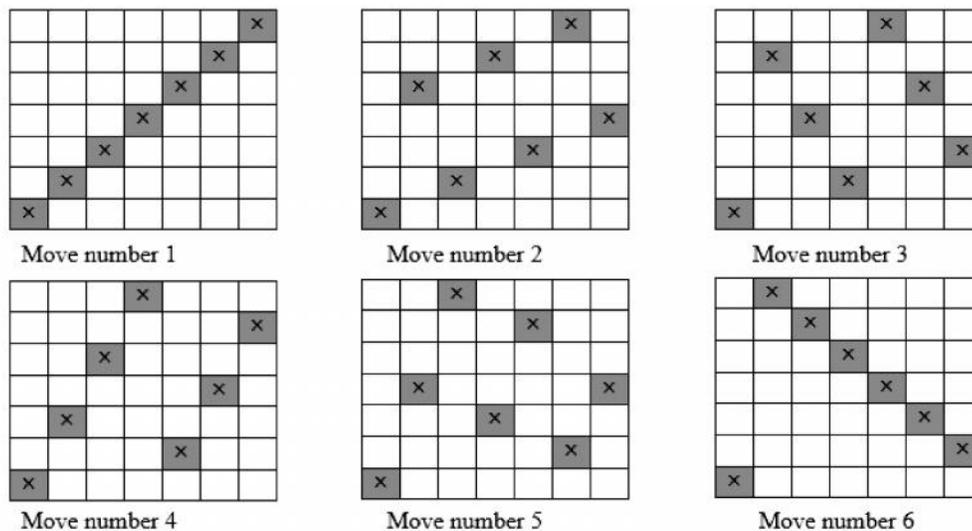
Figure 5.20: Seven-end sateen with various move numbers
