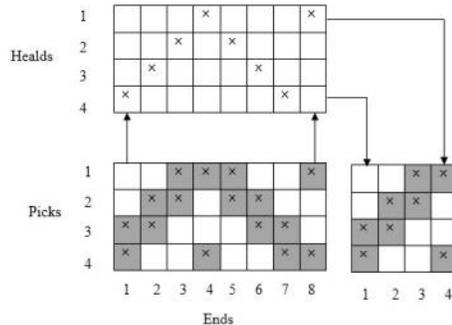
Figure 5.15: Design, drafting and lifting plan of pointed twill
