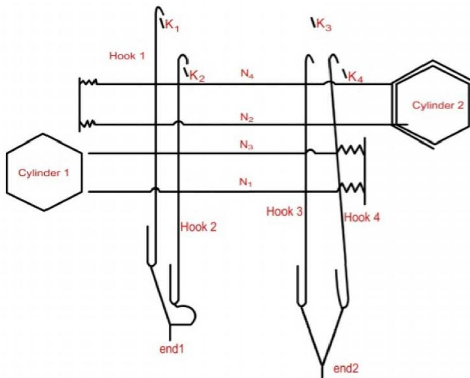
Figure 6.43: Side view of double-lift double-cylinder jacquard
