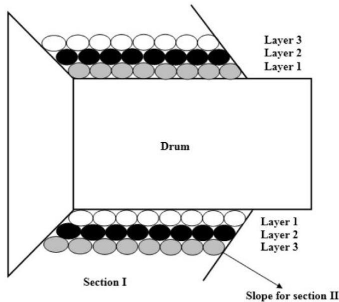
Figure 3.6: Schematic representation of sectional warping principle
