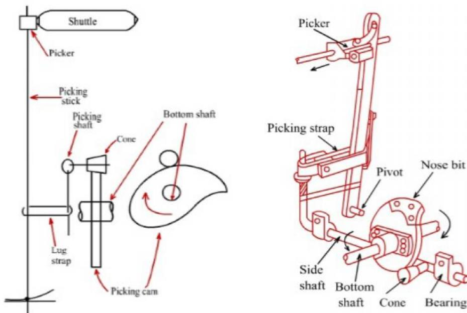
Figure 7.5: Cone under-pick mechanism
