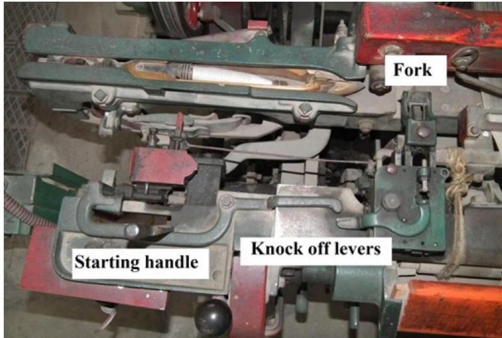
*Figure 9.15: Top view of side weft fork motion*
