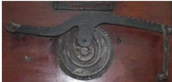
*Figure 6.4: A model of grooved cam*
