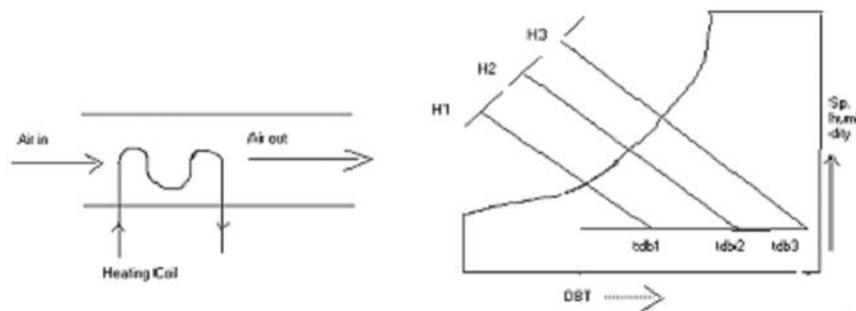
The bypass factor for the process is defined as the ratio of the difference between the mean surface temperature of the coil leaving the air temperature and the difference between the mean surface and the entering air temperature.
