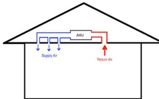
**SUPPLY DUCT CONFIGURATIONS** The configuration of a duct system is often like a tree with branches connected to the terminal units and a fan located at the root. In reality, the ductwork forms a double tree because the fan is in the middle of the supply and return/outside air parts of the system. The two most common supply duct systems are the ‘extended plenum’ system and the ‘radial’ system because of their versatility, performance, and economy.
