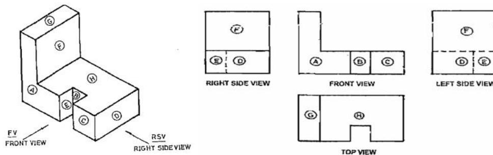
**Isometric projection:** The isometric projection of an object is a one plane view drawn with the object placed with respect to the plane of projection so that all the three principal axes appear to be inclined to each other at an equal angle of  $120^\circ$ .
