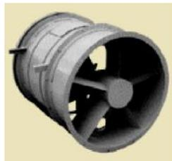
**Vaneaxial fans** are similar to tubeaxials, but with the addition of guide vanes that improve efficiency by directing and straightening the flow. As a result, they have a higher static pressure with less dependence on the duct static pressure. Such fans are used generally for pressures up to 500 mmWC. Vaneaxials are typically the most energy efficient fans available and
