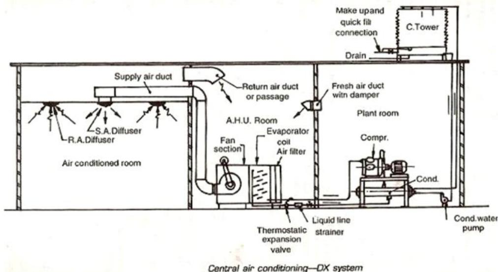
The plant room comprises of two important parts of the refrigeration system the compressor and the condenser. The compressor can either be of semi-hermetically sealed type or of open type. The semi-hermetically sealed compressor is cooled by air, which is blown by the fan, while the open type compressor is water-cooled. The open compressor can be driven directly by motor shaft by the coupling or by belt via pulley arrangement.
