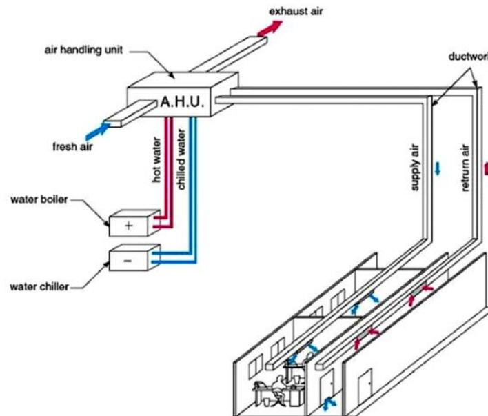
**Ductwork** is a branching network of round or rectangular tubes. It is generally constructed of sheet metal, fiberglass board, or a flexible plastic and wire composite material and is located within the walls, floors, and ceilings of the building.
