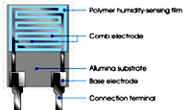
A thick film conductor of precious metals like gold, ruthenium oxide is printed and calcinated in the shape of the comb to form an electrode. Then a polymeric film is applied on the electrode; the film acts as a humidity sensing film due to the existence of movable ions. A change in impedance occurs due to the change in the number of movable ions.
