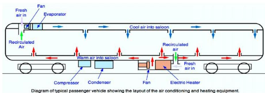
Passengers in a railway travel are adversely affected by infiltration of air unpleasantly laden with dust due to open windows. This is more so in the case of high speed passenger carrying trains. Secondly for a tropical country like India, the temperature varies from 46 degree C during summer to 2 degree C during winter. Airconditioning
