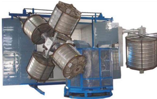
Fig: 3.4.5 Rotational Moulding machine
