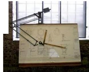
precisely adjusted with a controlling mechanism. There are two main types of apparatus: an arm-type parallelogram apparatus based on a hinged arm; and a track-type apparatus which moves on a rail mounted to the top of the drawing board. Small drafting machines (mini drafters) are commonly used.
