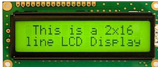
Along one side of a small printed board there are pins used for connecting to the microcontroller. There are in total of 14 pins marked with numbers (16 if the backlight is built in). Their function is described in the table below:
