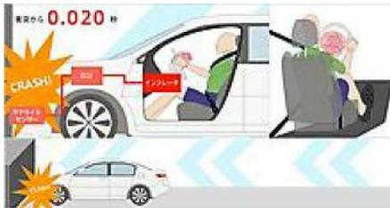
The inflators are activated through an igniter, causing a chemical reaction that emits gas, resulting in the deployment of the airbag cushion.
