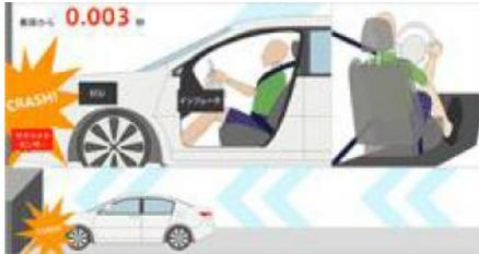
As the satellite sensors (collision sensors) attached to the vehicle detects the collision, a signal is sent to the ECU (Electronic Control Unit).
