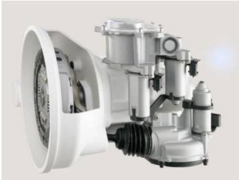
connection between the transmission and the selector lever. The transmission is controlled electronically through shift-by-wire.
