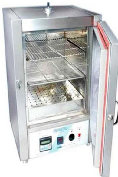
The hot air oven must not be opened until the temperature inside has fallen below 60°C to prevent breakage of glassware
