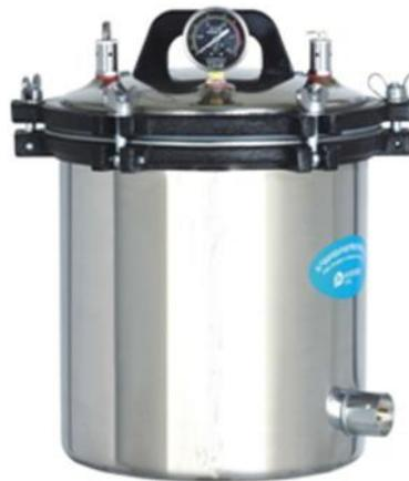
Articles sterilized by autoclaving are Culture media, dressings, linen etc. Autoclaving is the very effective method of sterilization, quicker than hot air oven. Drenching and wetting of articles, trapped air may reduce the efficacy, takes long time to cool are the disadvantages of the method.
