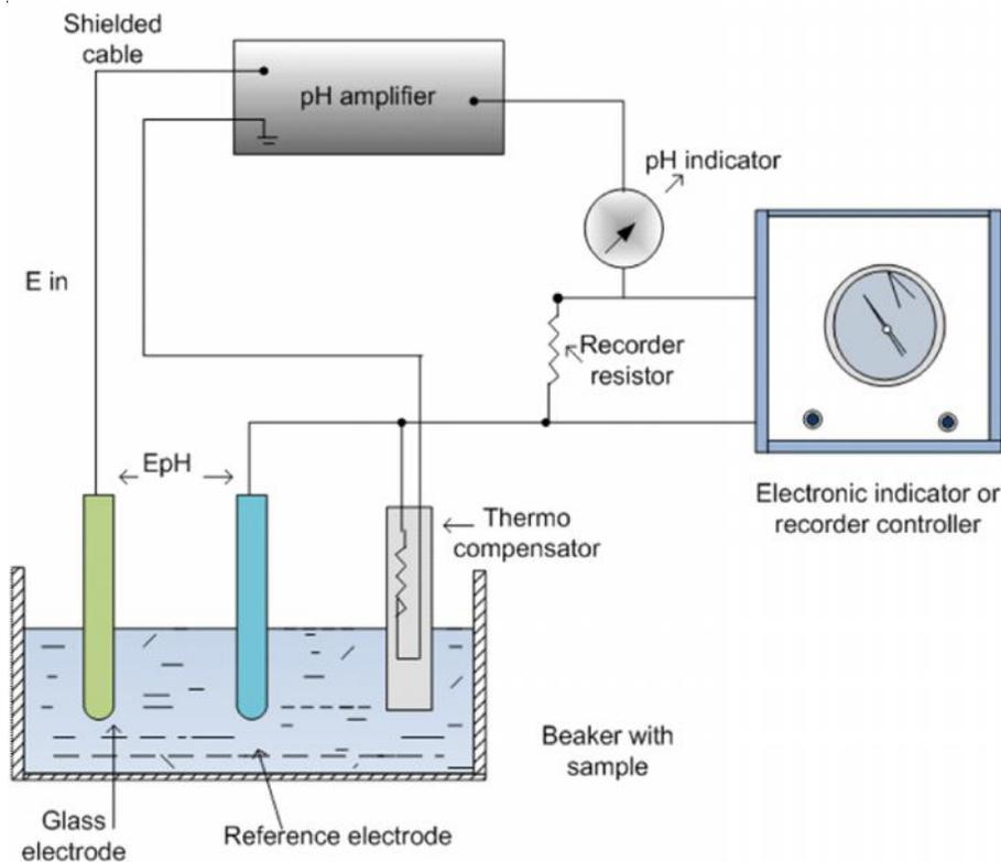
Circuit for electronic pH measurement
