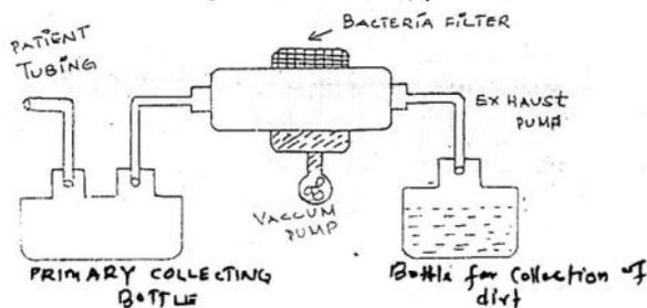
to create necessary vacuum for suction. By using tubing the fluids are sucked and primarily collected in a bottle, from there it is drawn to the bacteria filter or trap. This trap is connected in between the patient and vacuum inlet there for air is drawn in to the piping system. An exhaust is provided on the filter to remove the dirt collected in the trap.
