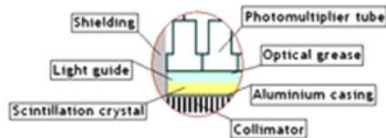
A gamma camera consists of one or more flat crystal planes (or detectors) optically coupled to an array of photomultiplier tubes in an assembly known as a "head", mounted on a gantry. The gantry is connected to a computer system that both controls the operation of the camera as well as acquisition and storage of acquired images. The construction of a gamma camera is sometimes known as a compartmental radiation construction.
