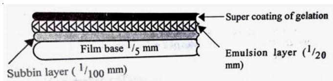
which silver bromide crystals are suspended uniformly. There are two layers of emulsion which are supported and separated by a polyester. This is called the film base. The
