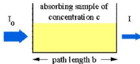
The Beer-Lambert law (or Beer's law) states that, when a monochromatic light passes through a solution, absorbance (A) of the solution is directly proportional to the concentration (c) of the solution and path length (b) of that solution. Now absorbance A is directly proportional to path length and concentration of that solution.
