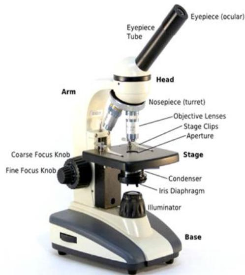
Eyepiece or Ocular is what you look through at the top of the microscope. Typically, standard eyepieces have a magnifying power of 10x. Optional eyepieces of varying powers are available, typically from 5x-30x.
