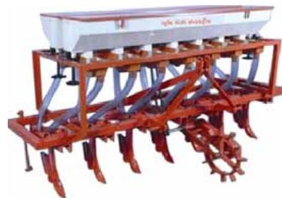
Seed - cum - fertilizer drills, fitted with fertilizer dropping attachment, distribute the fertilizer uniformly on the ground. The drill has a large seed box which is divided into 2 compartments one for seed and another for fertilizers. Seed drill can be bullock drawn or tractor drawn.
