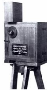
Fig1.7 (A) Cinematographe in camera mode
