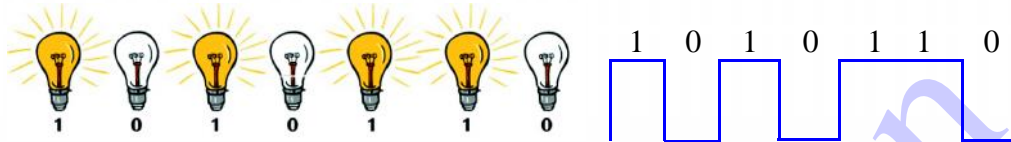
Fig. 1.8 : Digital representation of ON and OFF states
